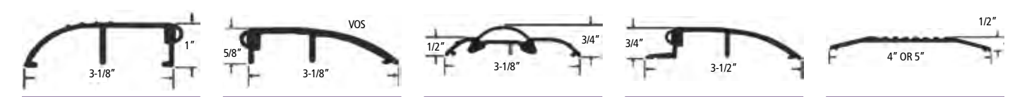
1" HIGH BUMPER HVOS Aluminum, Gold, Bronze, White 5/8" LOW BUMPER VOS Aluminum, Gold, Bronze, White 1/2" LOW SADDLE XLV Aluminum, Gold, Bronze, White 3/4" LOW BUMPER LIP SLV Aluminum, Gold, Bronze, White FLAT SADDLE 4" or 5" Aluminum
